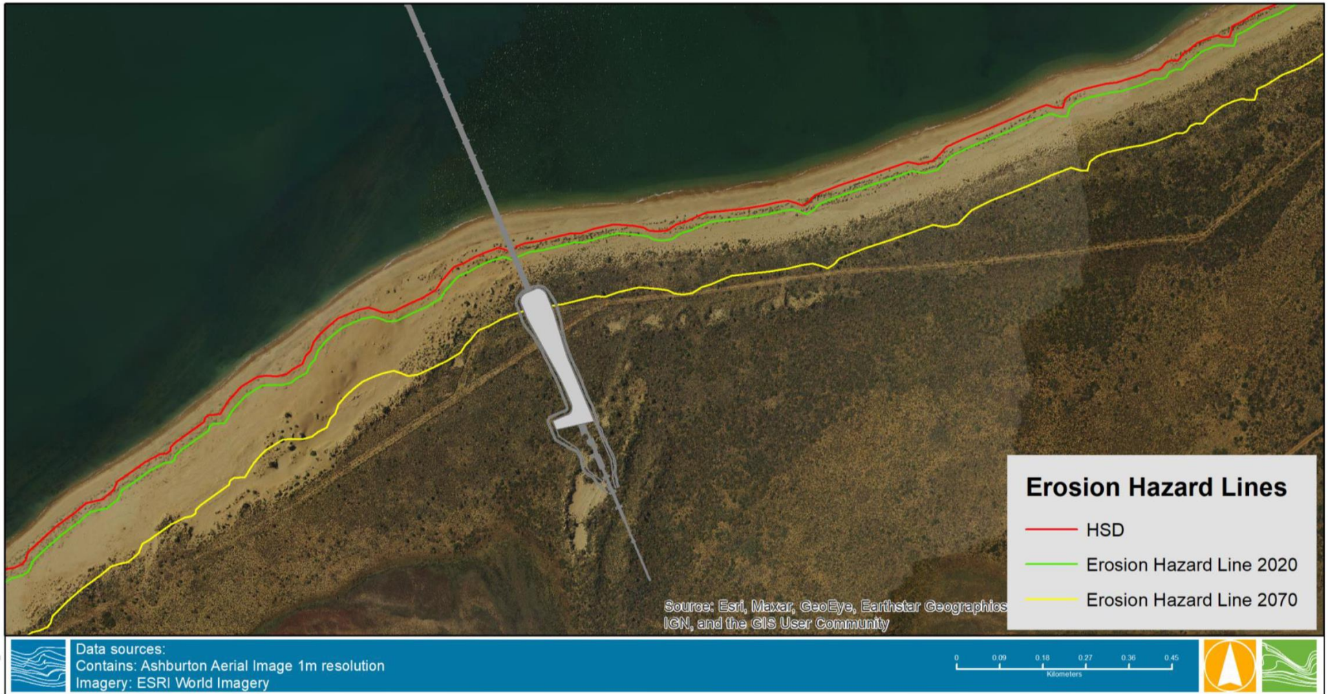
Figure 22: Coastal erosion hazard zone for 50-year design life, as per SPP2.6 methodology (HSD = Horizontal Shoreline Datum)
