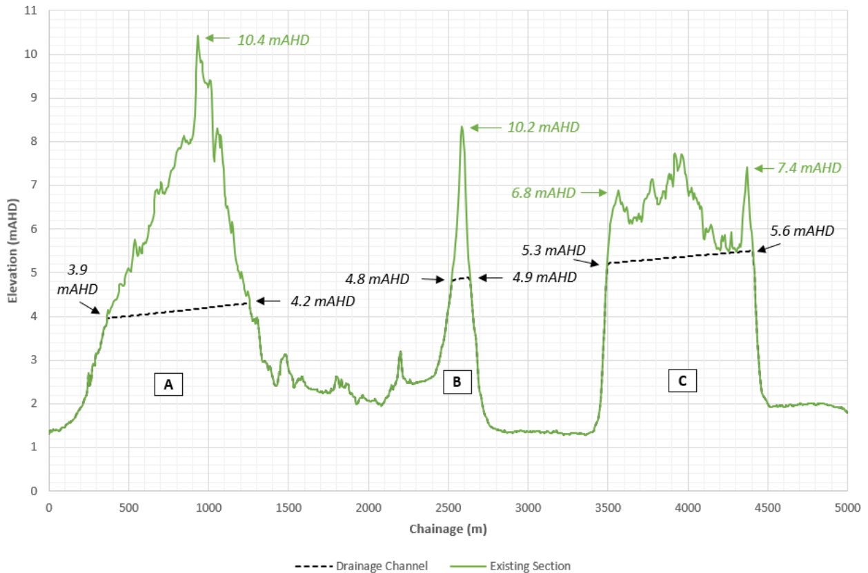
FIGURE 11-4 DIVERSION CHANNEL SECTION WITH ELEVATIONS
