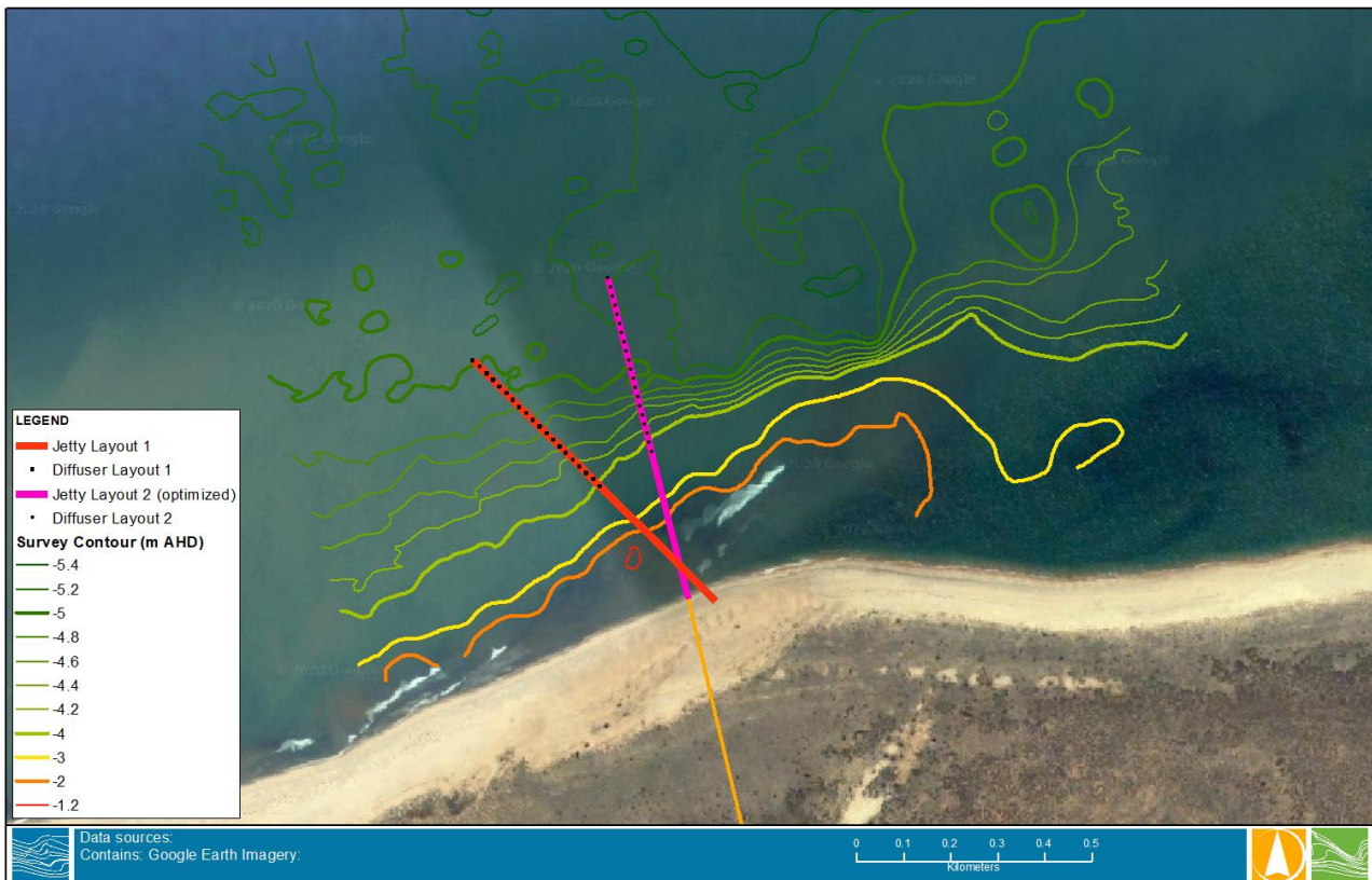
FIGURE 4-7 JETTY AND DIFFUSER LAYOUT OPTIMIZATION
