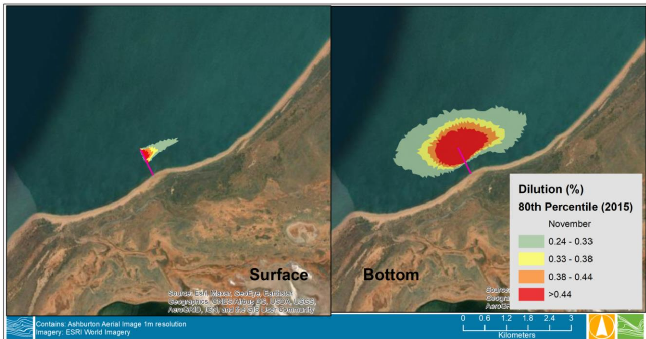
FIGURE 4-20 PREDICTED 80 TH PERCENTILE DILUTION AT THE SURFACE (LEFT) AND BOTTOM (RIGHT) FOR THE MONTH OF NOVEMBER
