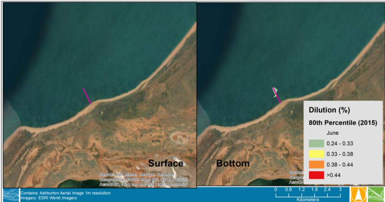
FIGURE 4-19 PREDICTED 80 TH PERCENTILE DILUTION AT THE SURFACE (LEFT) AND BOTTOM (RIGHT) FOR THE MONTH OF JUNE
